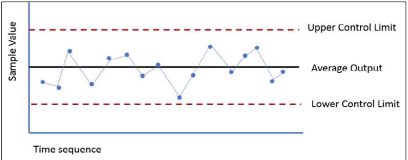
A basic descriptive SPC is now in place. Control charts can be applied to any process where data such as KPIs are available. The team, even if they are non-technical, understands this visual display of performance behavior. The gradual implementation of this process develops the team's analysis of the data to more focused and in-depth discussions.
